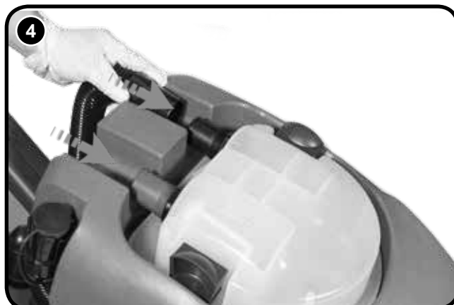
Fit both vacuum and floor-tool hose to the separator (Fig.4).
